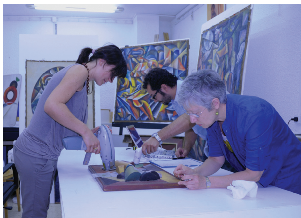
I. Cassan using an XRF (left). Denis Pitzalis (Scientific Researcher at the Cyprus Institute / Centre de Recherche et Restauration des Musées de France) using a video microscope (centre). Laurette Thomas taking a sample (right).
